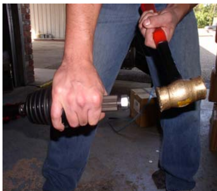
Axle Nut on Shaft. Drive Axle into Diff. at slight angle
